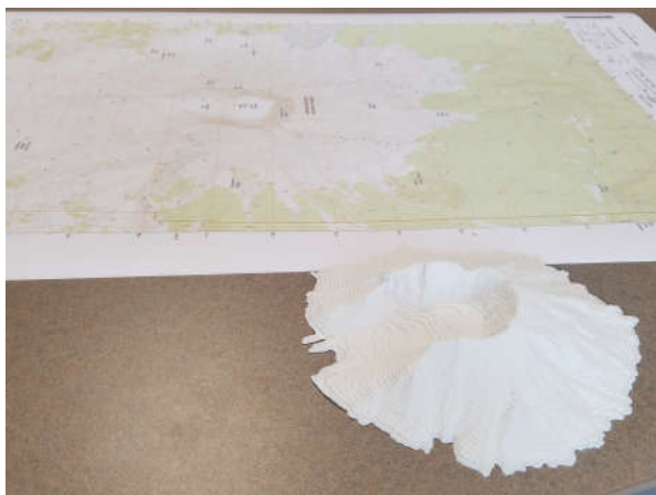
3D printed model of Mount Saint Helens with corresponding USGS Quadrangle. Credit: Ashley Coles
